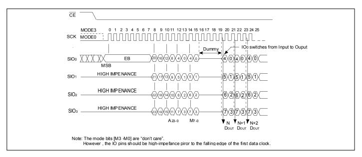
Figure 8: Fast Read Quad I/O Sequence ([M7-M0] = 0xH or NOT AxH)
