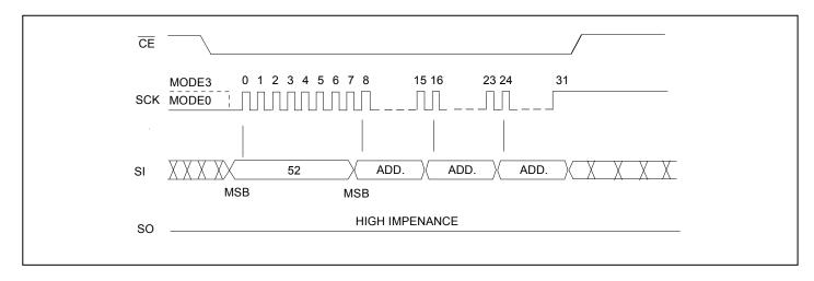
Figure 14: 32K-byte Block Erase Sequence
