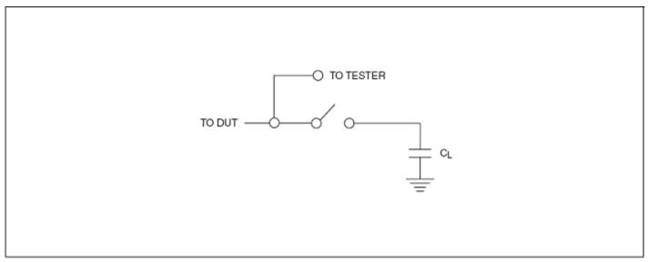
Figure 35: A Test Load Example
