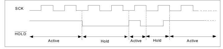
Figure 1: HOLD Condition Waveform
