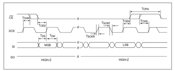
Figure 29: Serial Input Timing Diagram
