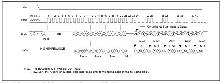
Figure 5: Fast Read Dual I/O Sequence ([M7-M0] = 0xH or NOT AxH)
