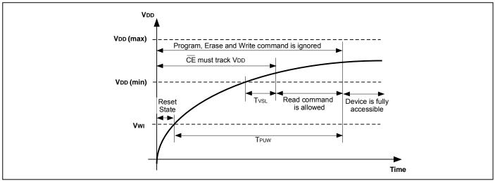
Figure 33: Power-Up Timing Diagram
