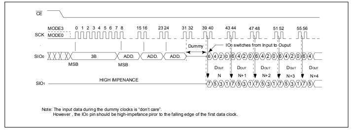
Figure 4: Fast Read Dual Output Sequence
