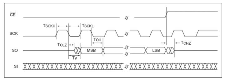
Figure 30: Serial Output Timing Diagram
