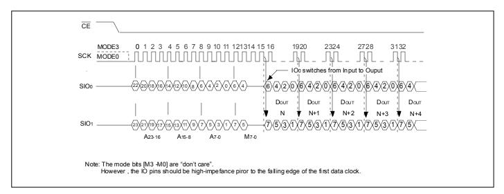
Figure 6: Fast Read Dual I/O Sequence ([M<sub>7</sub>-M<sub>0</sub>] = AxH)
