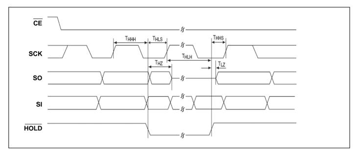
Figure 31: HOLD Timing Diagram
