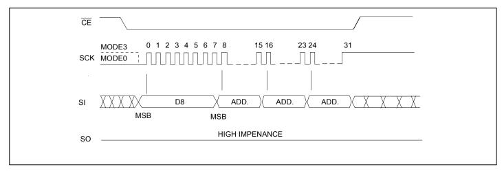
Figure 13: 64K-byte Block Erase Sequence
