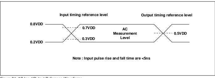
Figure 34: AC Input/Output Reference Waveforms
